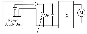
Add the zener diode in parallel with bypass capacitance
