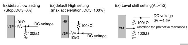
Since the resistance value is a reference value, please change according to the operating conditions. In addition, the input voltage of the VSP terminal ask attention to the absolute maximum rating. It should be noted that, If you connect a resistor to the HB terminal, please set the resistance value with attention to the rated current of the HB terminal.
